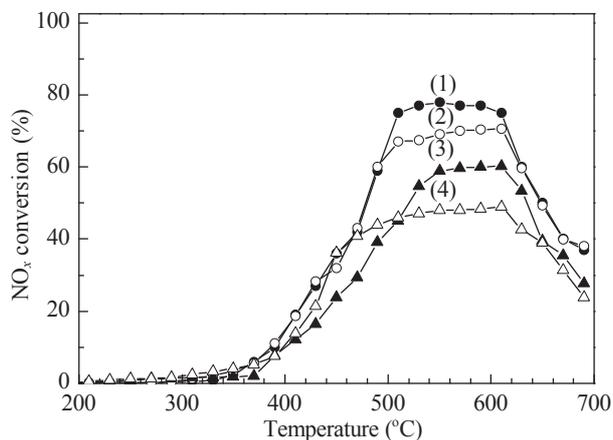
**Fig. 6.** Effect of space velocity on the  $NO_x$ -SCR activity of Cu-SAPO-34/cordierite. Space velocity: (1)  $3000\ h^{-1}$ ; (2)  $4000\ h^{-1}$ ; (3)  $6000\ h^{-1}$ ; (4)  $12000\ h^{-1}$ . Reaction conditions: 0.05%  $NO_x$ , 0.05%  $C_3H_8$ , and 7%  $O_2$ .
