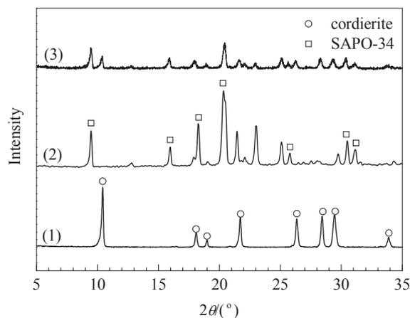
**Fig. 1.** XRD patterns of black cordierite (1), Cu-SAPO-34 (2), and Cu-SAPO-34/cordierite (3).
