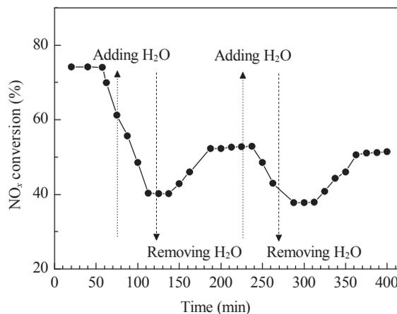
**Fig. 8.** Effect of  $H_2O$  on the  $NO_x$  concentration of the effluent in Cu-SAPO-34/cordierite. Reaction conditions: 0.05%  $NO_x$ , 0.05%  $C_3H_8$ , 7%  $O_2$ , 10%  $H_2O$  (when used),  $SV = 3000\ h^{-1}$ , and  $500\ ^\circ C$ .
