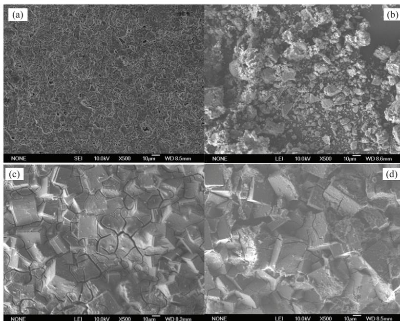
**Fig. 2.** SEM images of the surface of blank cordierite (a), Cu-SAPO-34/cordierite powder (b), external surface (c), and internal surface (d) of Cu-SAPO-34/cordierite.
