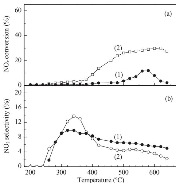
**Fig. 3.**  $\text{NO}_x$  conversion (a) and  $\text{NO}_2$  selectivity (b) of SAPO-34/cordierite (1) and Cu-SAPO-34/cordierite (2). Experimental conditions:  $0.05\% \text{ NO}_x$ ,  $0.05\% \text{ C}_3\text{H}_8$ ,  $7\% \text{ O}_2$ , and  $\text{SV} = 6000 \text{ h}^{-1}$ .
