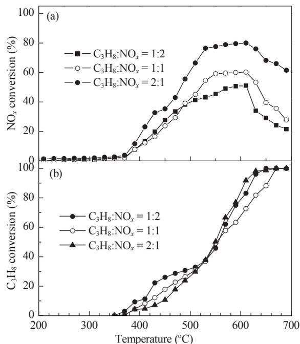
**Fig. 4.** Effect of  $\text{C}_3\text{H}_8/\text{NO}_x$  ratio on the  $\text{NO}_x$ -SCR activity of Cu-SAPO-34/cordierite. Experimental conditions:  $0.05\% \text{ NO}_x$ ,  $7\% \text{ O}_2$ ,  $\text{C}_3\text{H}_8/\text{NO}_x = 1:2, 1:1$  or  $2:1$ , and  $\text{SV} = 3000 \text{ h}^{-1}$ .
