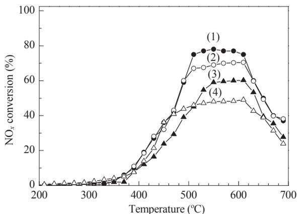
**Fig. 5.** Effect of  $O_2$  concentration on the  $NO_x$ -SCR activity of Cu-SAPO-34/cordierite.  $O_2$  concentration: (1) 2%; (2) 5%; (3) 7%; (4) 10%. Experimental conditions: 0.05%  $NO_x$ , 0.05%  $C_3H_8$ , and  $SV = 3000\ h^{-1}$ .
