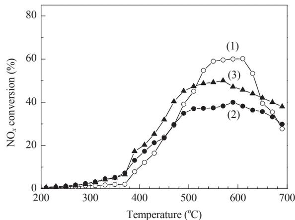
**Fig. 7.** Effect of water vapor on the  $NO_x$ -SCR activity of Cu-SAPO-34/cordierite. (1) Before adding water; (2) Adding water; (3) Stop adding water. Experimental conditions: 0.05%  $NO_x$ , 0.05%  $C_3H_8$ , 7%  $O_2$ , and  $SV = 3000\ h^{-1}$ .
